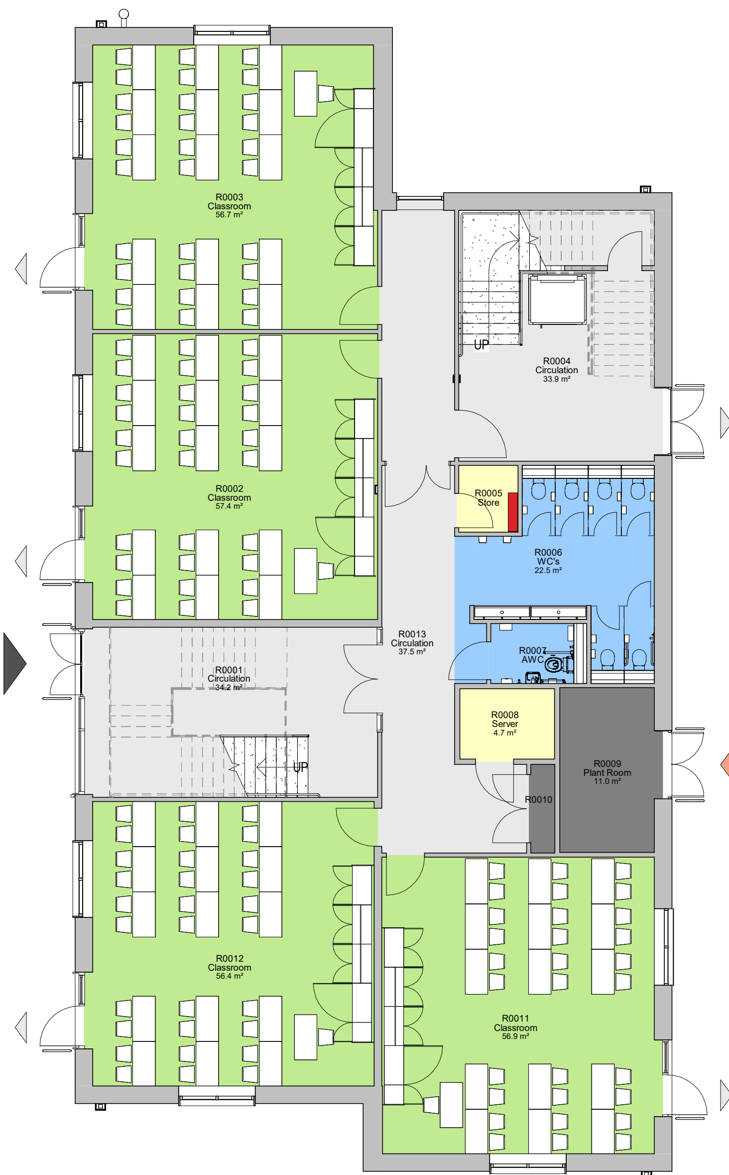
1 Ground Floor General Arrangement Plan 1 : 100
